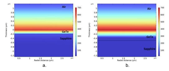
Figure 80. Temperature distribution inside the GeTe layer at the time of peak temperature at its surface for a green laser ( $\lambda$  = 532 nm) and a fluence of 10 mJ/cm², for a) 200-nm thick layer and b) 500-nm thick layer.
