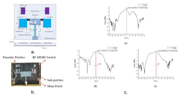
Figure 13. Radiation pattern reconfigurable antenna using two RF-MEMS switches. a) Schematic representation. b) Fabricated antenna with integrated RF-MEMS switches. c) Measured radiation pattern in the three states. From [25].
