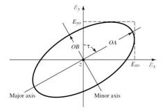
Figure 164. Polarization ellipse. Adapted from [11]
