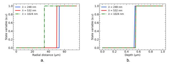
Figure 76. a) Amorphous-to-crystalline state variable distribution over the surface of the GeTe layer at the end of the simulation. b) State variable distribution in the depth of the GeTe layer at the end of the simulation. (S = 0 for crystalline GeTe and S = 1 for amorphous state).
