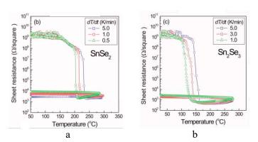
Figure 23. Surface resistance evolution with temperature for different heating rates of a 90 nm thin film of a) SnSe<sub>2</sub> and b) Sn<sub>2</sub>Se<sub>3</sub>. From [46].
