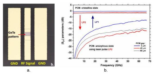
Figure 44. a) Fabricated of a simple GeTe RF-switch without heater. b) Measured performance of both states after laser irradiation for different GeTe gaps [80].
