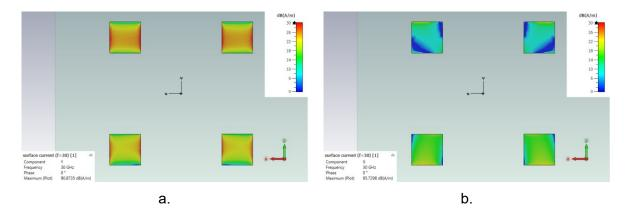
Figure 103. Surface current densities on the array antennas using an alumina superstrate for a separation of  $\lambda/2.25$ . a) Magnitude of  $J_{\gamma}$ . b) Magnitude of  $J_{\chi}$ .
