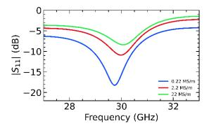
Figure 142. Simulated influence of the metal conductivity in the S-parameters of the RHCP antenna.
