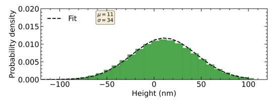
Figure 101. Measured histogram and fitter gauss bell curve of the surface profile of an alumina substrate.
