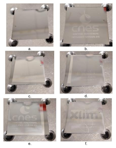
Figure 95. Writing and erasing procedure of arbitrary shapes in a GeTe layer. a) As-deposited 250-nm GeTe layer on a 25x 25 mm² sapphire substrate. b) Writing of an arbitrary shape using laser engraving (CNES logo-crystalline). c) Erasing of the previously written pattern by crystallizing the whole pattern d) Amorphization of the whole written surface. e) Re-write of the CNES logo (crystalline) d) Erasing and writing of another arbitrary pattern in the surface (XLIM logo-amorphous).
