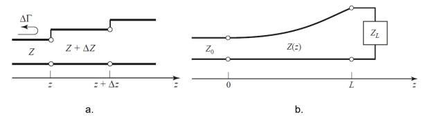
Figure 122. a) Model of an impedance step change. b) Model of a smooth change in impedance using a taper line.
