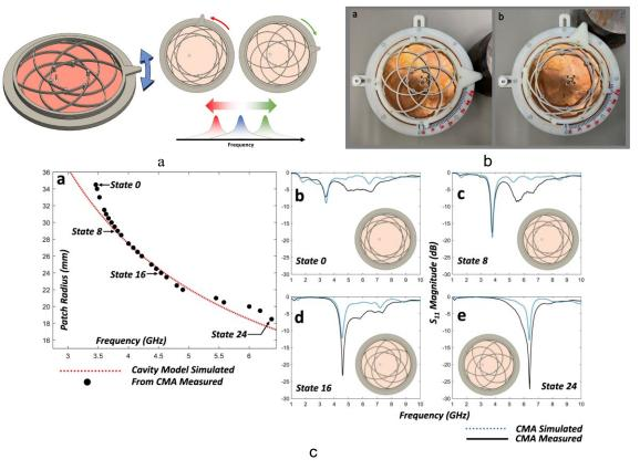
Figure 6. Mechanically reconfigurable antenna with continuous tuning of the operation frequency.
