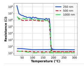
Figure 48. Evolution of the surface resistance as a function of temperature of a 250-nm, 500-nm and 1000 nm-thick layers of GeTe obtained on a c-cut (0001) sapphire substrate.
