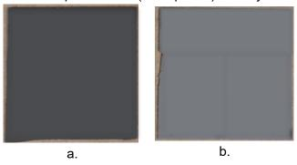
Figure 50. Optical images of a 250-nm layer of GeTe deposed over a 25x25 mm<sup>2</sup> sapphire substrate in a) amorphous state and b) crystalline state.
