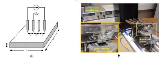
Figure 51. a) Schematic representation of the 4-point probe technique to extract the conductivity of thin films. b) Measurement system employed to measure the conductivity of the film.
