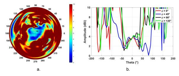
Figure 153. Measured axial ratio of a full-metal LHCP array of antennas at 29.6 GHz. a) Full picture. b) At planes  $\varphi = 0$ , 45, 90 and 135°.
