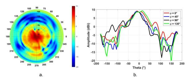
Figure 147. Measured directivity of a full-metal RHCP array of antennas at 29.6 GHz. a) Full picture. b) Directivity at planes  $\varphi = 0$ , 45, 90 and 135°.
