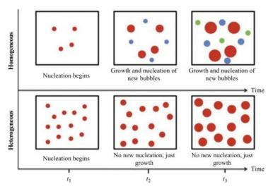
Figure 22. Time diagram of homogeneous and heterogenous nucleation. At time  $t_1$ , crystals begin to form within the material in random positions due to nucleation. At time  $t_2$ , for homogenous nucleation, new crystal clusters begin to form by nucleation while the previously formed clusters grow in size. At time  $t_3$  the crystal clusters have grown significantly in size while the nucleation and crystal growth continues until the whole material is crystalline. Taken from [47].
