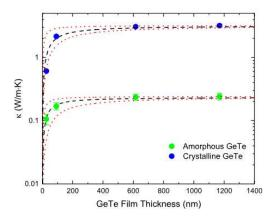
Figure 34. Measured thermal conductivity of an amorphous and crystalline GeTe samples for various thickness samples. From [71].
