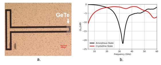
Figure 62. a) Fabricated quarter-wavelength stub resonator on a sapphire substrate with a 500-nm thick GeTe pattern at the end of the resonator. b) Measured transmission of the resonator at both states of the GeTe pattern.
