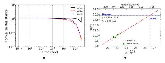
Figure 53. a). Stress acceleration test on three samples of GeTe deposited on a sapphire substrate. b) Linear plot of the Arrhenius equation showing the crystallization time of the accelerated temperature stress test on the three samples.
