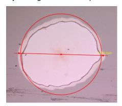
Figure 88. Crystallized area by a single 480-µJ laser pulse on a 500-nm thick GeTe layer deposited over a sapphire substrate.
