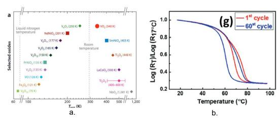
Figure 18. a) Examples of phase transition materials and the associated transition temperatures [38]. b) Variation of the normalized resistivity of a VO<sub>2</sub> film during a heating - cooling cycle [39].
