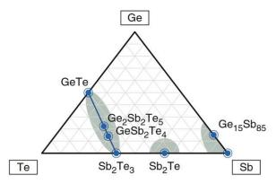
Figure 29. Diagram showing some of the most common (and studied) PCM compositions of the ternary Ge-Sb-Te for RF applications [33].
