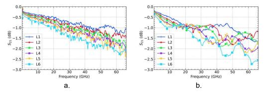
Figure 65. a) Measured S<sub>21</sub> parameters of all the CPW lines fabricated on an alumina substrate integrating a thin layer of a 500-nm thick GeTe (sample 2) and b) similar parameters of the CPW lines fabricated on a SiO<sub>2</sub> substrate integrating a thin layer of a 800-nm thick GeTe (sample 3).
