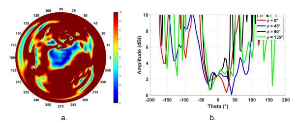
Figure 151. Measured axial ratio of a full-metal LHCP array of antennas at f = 30 GHz. a) Full picture. b) At planes  $\phi = 0$ , 45, 90 and 135°.
