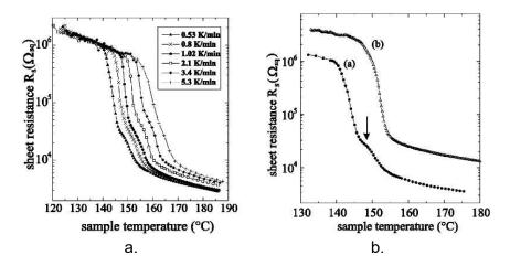
Figure 37. a) Surface resistance evolution of 80-nm thin film. b) Surface resistance evolution for a 80-nm GST thin film covered by a 4.5-nm ZnS-SiO<sub>2</sub> capping layer. From [76].
