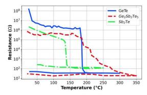
Figure 49. Evolution of the surface resistance as a function of temperature of a GeTe, GST and Sb<sub>2</sub>Te PCM compositions obtained on a c-cut (0001) sapphire substrate.
