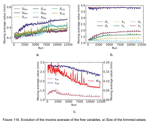
Figure 116. Evolution of the moving average of the free variables. a) Size of the trimmed edges. b) Size of the of the antennas and the array. c) Size of the coupling slot.
