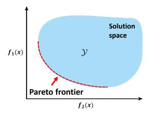
Figure 112. Graphical representation of a pareto frontier of the solution space for a two-objective optimization.
