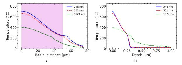
Figure 75. a) Temperature distribution over the surface of the GeTe layer at the time of peak temperature for different wavelengths (the violet shaded area represents the laser beam radius).
