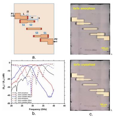
Figure 47. a) Schematic representation of the parallel coupled half-wavelength filter b) Measured S-parameters of the filter in both states of the GeTe. c) Optical images of the filter integrating a GeTe pattern in the amorphous state (upper-half) and in crystalline state (lower-half). From [88].
