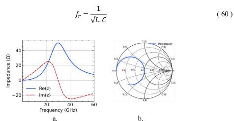
Figure 160. Evolution of the input impedance of a parallel RLC circuit as a function of frequency.
