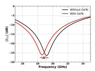
Figure 64. Measured S<sub>21</sub> parameter of a stub resonator with length of 1.3 mm showing clear changes in the parallel resonant frequency due to the addition of a 500-nm thick layer of GeTe.
