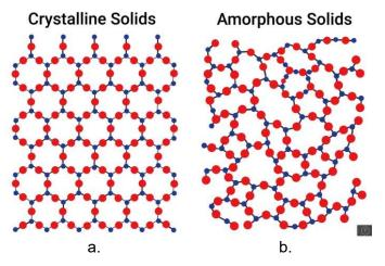
Figure 20. Illustration of the atomic arrangement of a a) crystalline solid and b) amorphous solid.
