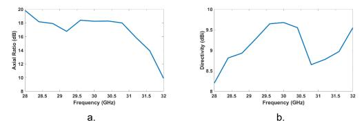
Figure 158. Measured far-field performances of the array of antenna shown in Figure 155 after crystallizing the remaining amorphous GeTe patterns. a) Axial ratio in the axis and, b) Maximal directivity
