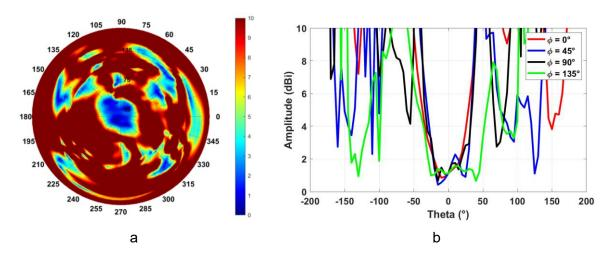
Figure 148. Measured axial ratio of a full-metal RHCP array of antennas at 30 GHz. a) Full picture. b) At planes  $\varphi = 0$ , 45, 90 and 135°.
