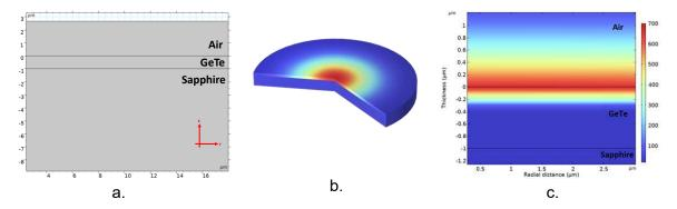
Figure 73. a) COMSOL geometry of a PCM (GeTe) layer over a sapphire substrate. b) Spatial distribution of the laser beam. C) 2D heating profile of a 1-µm thick GeTe sample.
