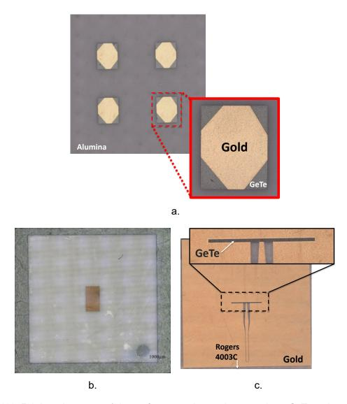
Figure 130. Fabricated antenna. a) Array of antennas integrating amorphous GeTe at the top of the alumina substrate. b) Exciter antenna at the top of the ROGERS 4003C substrate (The dark dot at the bottom right is an ink marker for orientation purposes). c) Ground planes, input transmission line and slot window integrating amorphous GeTe.
