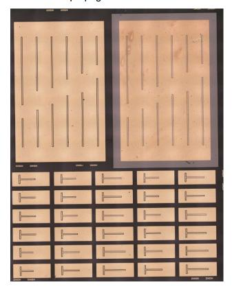
Figure 60. Complete image of the all the fabricated CPW lines over a layer of alumina (upper left) and over a layer of GeTe/alumina (upper right) and all the fabricated stub resonators with and without a layer of GeTe (the bonding of the resonators is not shown).
