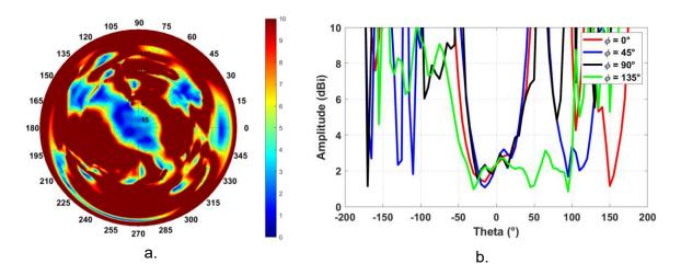
Figure 150. Measured axial ratio of a full-metal RHCP array of antennas at 29.6 GHz. a) Full picture. b) At planes  $\varphi = 0$ , 45, 90 and 135°.
