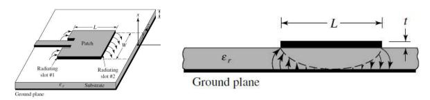
Figure 3. Example of a planar rectangular antenna (microstrip antenna). a) Full view. b) Side view. Taken from [24].
