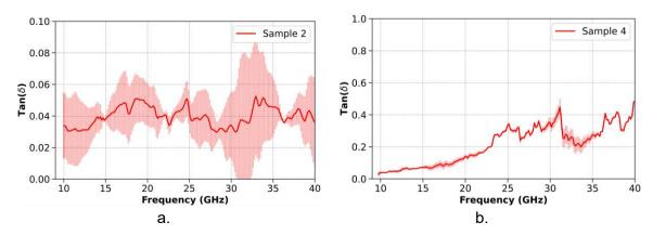
Figure 70. a) Mean and dispersion values of the extracted loss tangent of the GeTe from sample 2 and, b) of the GST from sample 4.
