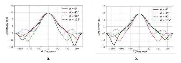
Figure 119. Simulated directivity at four cuts on the  $\Phi$  plane for the current best configuration. a) RHCP antenna b) LHCP antenna.
