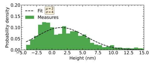
Figure 100. Measured histogram and fitted curve of the surface profile of a quartz substrate.
