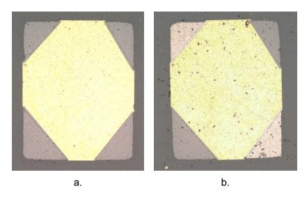
Figure 155. Examples of the new fabricated array of antennas using a lift-off technique.
