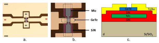
Figure 40. Example of a GeTe-based PCM-switch. a) Fabricated device. b) Close up to the GeTe composition. c) Schematic representation of the different layers of the circuit. From [81].
