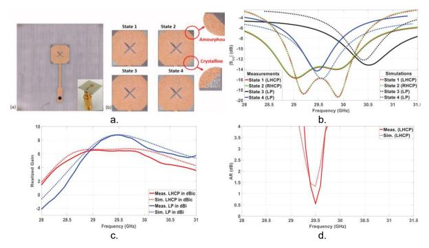
Figure 45. Optically activated planar antenna integrating a GeTe composition for polarization reconfiguration. a) Fabricated device. b) Measured S<sub>11</sub> performance in all states. c) Simulated and measured realized gain in LHCP and LP state. d) Simulated and measured axial ratio in LHCP state. From [81].
