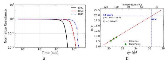
Figure 54. a). Stress acceleration test on three samples of Sb<sub>2</sub>Te deposited on a sapphire substrate. b) Linear plot of the Arrhenius equation showing the crystallization time of the accelerated temperature stress test on the three samples.
