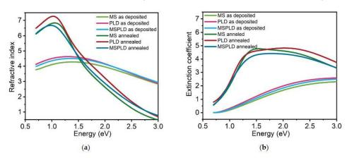
Figure 39. Measured influence of the deposition method on the optical properties of a 30-nm GST film for amorphous (as deposited) and crystalline state (annealed) [74].
