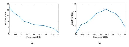
Figure 156. Measured far-field performances of the array of antennas after optical irradiation (as shown in Figure 155). a) Axial ratio in the axis and, b) Maximal directivity.
