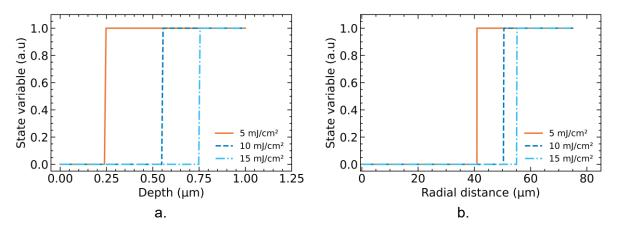
Figure 77. a) State variable distribution over the depth of the GeTe layer for different energy densities for  $\lambda = 532$  nm. b) State variable distribution over the surface of the GeTe layer for different energy densities for  $\lambda = 532$  nm. (S = 0 for crystalline GeTe and S = 1 for amorphous state).
