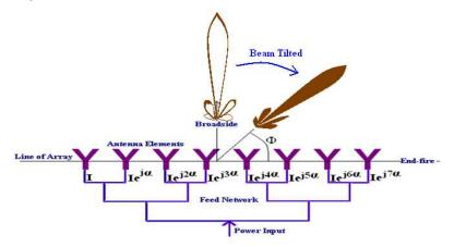
Figure 5. Example of a steerable beam using a linear array of antennas. From [17].
