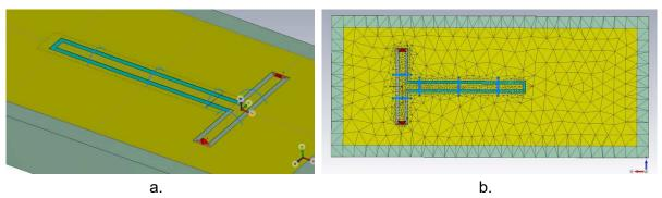
Figure 63. a) 3D electromagnetic model of an open-circuit stub resonator integrating a thin line of GeTe and bonding wire over an alumina substrate. b) Tetrahedral mesh of the stub resonator.
