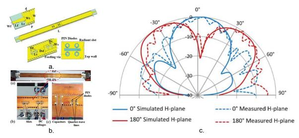
Figure 10. Radiation pattern reconfigurable SIW antenna using PIN diodes. a) Schematic representation. b) Fabricated SIW antenna with integrated diodes. c) Radiation pattern for two configurations. From [21].
