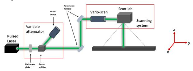
Figure 81. Diagram of the complete optical irradiation set-up.
