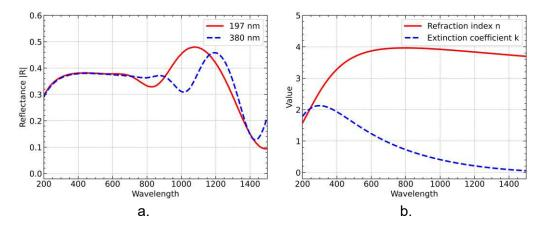
Figure 72. a) Measured reflectance of two samples of GeTe over a sapphire substrate. b) Extracted refraction index and extinction coefficient for the 197-nm thick sample.
