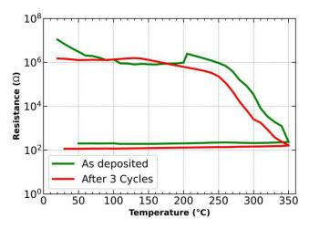
Figure 94. Evolution of the surface resistance of a GeTe layer as a function of temperature after 3 complete cycles of optical induced crystallization-amorphization.
