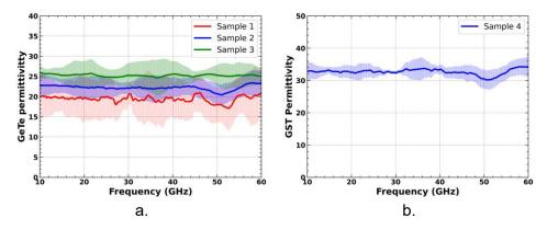
Figure 68. a) Mean and dispersion values of the extracted permittivity of GeTe using the analytical method for all samples integrating GeTe (samples 1 to 3). b) Mean and dispersion values of the extracted GST permittivity using the analytical method.
