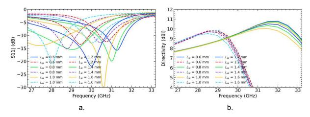
Figure 128. Performance linearly polarized configuration as the effective length of the slot is changed when all GeTe edges are in the crystalline state (dashed lines) and all the GeTe edges are in the amorphous state (solid lines). A) S-parameters b) Directivity.
