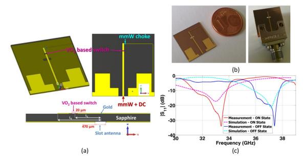
Figure 19. Frequency reconfigurable antenna integrating VO<sub>2</sub> for mmWave frequencies. a) Schematic representation of the antenna design. b) Fabricated device. c) Measured and simulated operation frequency in both states of the VO<sub>2</sub> switch. From [40].
