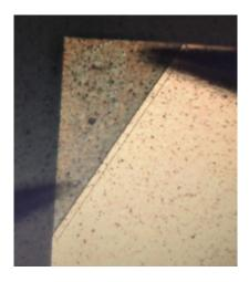
Figure 154. Optical image of the irradiated GeTe edge of the array of antennas. The black features are the out-of-focus probes.
