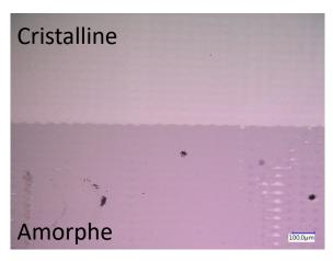
Figure 93. Amorphized area of a 250-nm thick GeTe sample using laser irradiation of a previously crystallized zone.
