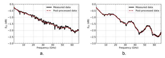
Figure 66. a) Measured S<sub>21</sub> parameters of the L<sub>6</sub> line in sample 2 (alumina substrate) with a thin layer of GeTe before and after post-processing filter and b) similar result for the L<sub>6</sub> CPW line with a thin layer of GeTe on sample 3 (SiO<sub>2</sub> substrate).
