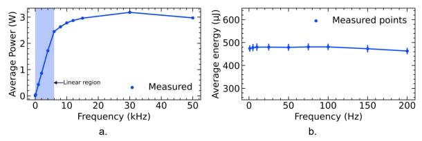
Figure 86. a) Average power of the laser measured over the whole frequency range. b) Average energy of the laser measured up to 200 Hz.
