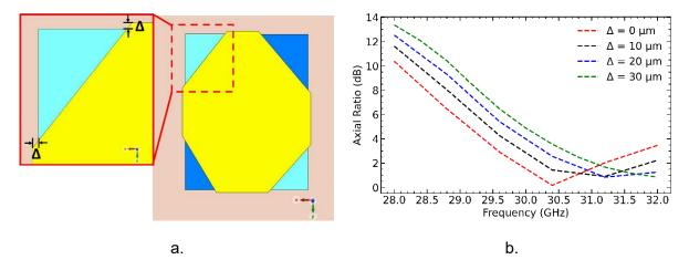
Figure 157. Simulation of the perturbation effect on the axial ratio of a RHCP antenna from a misalignment of the GeTe pattern. a) Geometry of the perturbation. b) Simulated axial ratio.
