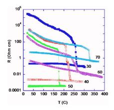
Figure 30. Evolution of the surface resistance of a Ge-Te alloy for various compositions [62].
