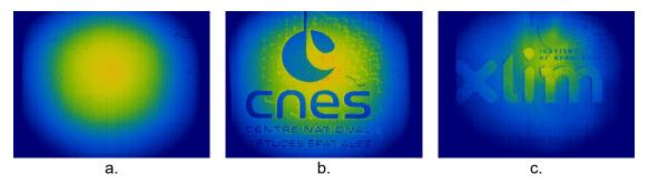
Figure 96. Thermal infrared images of the a) As deposited 250-nm thick GeTe layer. b) After engraving the CNES logo. c) After erasing the previously written CNES logo and re-writing the XLIM logo.
