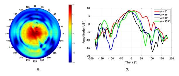
Figure 145. Measured directivity of the LP (all GeTe edges in amorphous state) array of antenna at 29.6 GHz. a) Full picture. b) Directivity at planes  $\varphi = 0$ , 45, 90 and 135°.
