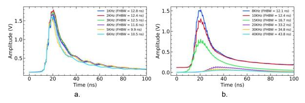
Figure 87. Measured temporal pulse shape of the pulsed laser source in the a) linear region and, b) saturated region.
