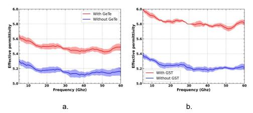
Figure 67. a) Comparison of the mean effective permittivity values extracted using the TRL method from the fabricated CPW lines on an alumina substrate, with and without a GeTe layer of 800 nm (sample 2). b) Comparison of the mean effective permittivity, with and without a GST layer of 800 nm (sample 4).
