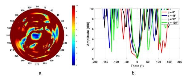
Figure 152. Measured axial ratio of a full-metal LHCP array of antennas at 30.4 GHz. a) Full picture. b) At planes  $\varphi = 0$ , 45, 90 and 135°.
