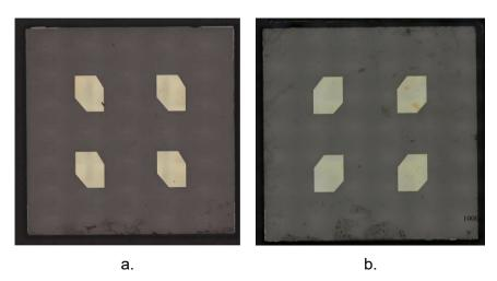
Figure 131. Fabricated full metallic array of antennas. a) RHCP array. b) LHCP array.
