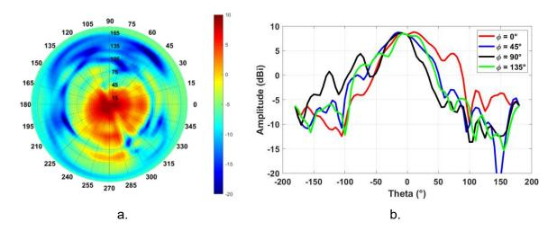
Figure 146. Measured directivity of a full-metal LHCP array of antennas at 29.6 GHz. a) Full picture. b) Directivity at planes  $\varphi = 0$ , 45, 90 and 135°.
