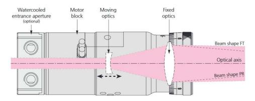
Figure 85. Schematic representation of the VarioScan system.
