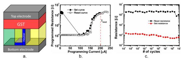
Figure 26. a) Schematic representation of a memory PCM cell. b) Resistance of the cell as a function of programming current. c) Resistance variation as a function of number of cycles. Taken from [52].
