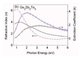
Figure 38. Measured optical properties of a sample of GST in amorphous (blue trace) and crystalline state (black trace) [68].
