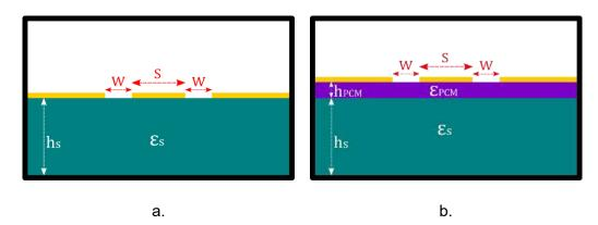
Figure 56. a) Cross-section of the geometry of a CPW in a bare substrate. b) Cross-section of the geometry of a CPW integrating a PCM thin film on a substrate.
