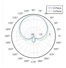
Figure 163. Normalized radiation pattern of a patch antenna.
