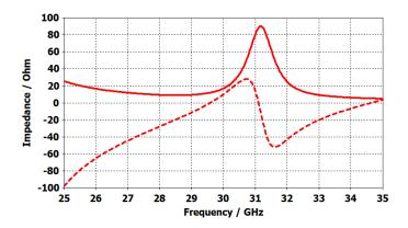
Figure 125. Simulated behavior of input impedance of the matched antenna using the proposed matching network in for a L<sub>w</sub> = 0.6 mm.
