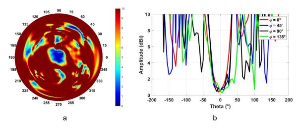
Figure 149. Measured axial ratio of a full-metal RHCP array of antennas at 30.4 GHz. a) Full picture. b) At planes  $\varphi = 0$ , 45, 90 and 135°.
