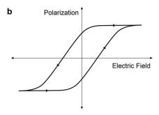
Figure 16. Typical variation of the dielectric polarization in a ferroelectric material as a function of the applied electric field.
