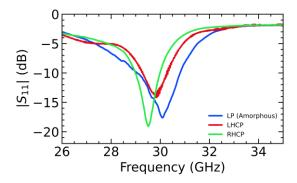
Figure 137. Comparison of the measured matching performance of the three states of polarization with a ROGERS 4003C substrate.
