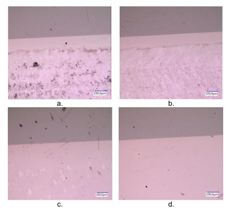
Figure 91. Crystallized zone of a 250-nm thick GeTe layer for a laser power attenuation factor of a) 100% transmission ( $E_{pulse}$  = 450  $\mu$ J), b) 50% transmission ( $E_{pulse}$  = 225  $\mu$ J), c) 20% transmission ( $E_{pulse}$  = 90  $\mu$ J) and d) 5% transmission ( $E_{pulse}$  = 22.5  $\mu$ J).
