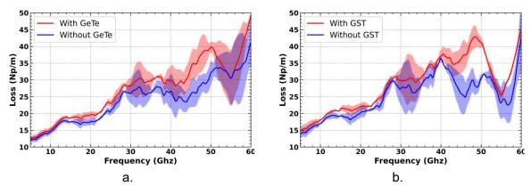
Figure 69. a) Comparison of the mean losses values extracted using the TRL method from a fabricated transmission line on alumina substrate with and without a GeTe layer of 800 nm (sample 2) and, b) for a fabricated transmission line on alumina substrate with and without a GST layer of 800 nm (sample 4).
