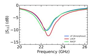
Figure 140. Comparison of the measured matching performance of the three states of polarization with a quartz substrate with a ground plane with a slot window of  $L_w = 2.4$  mm.
