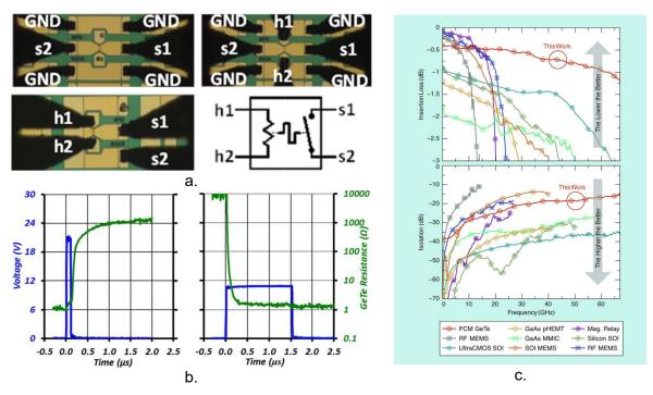
Figure 42. a)Layout of the proposed GeTe-based RF switch. b) Measured switching time of the amorphization (left) and crystallization (right) of a GeTe-based switch 0.9 µm length. c) Comparison of insertion loss in the ON state and isolation in the OFF state of PCM switches against other switching technologies.
