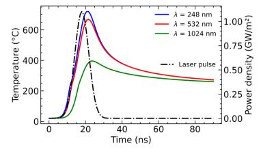
Figure 74. Simulation results of the evolution of the surface temperature in a 1-µm thick layer of GeTe for multiple wavelengths with energy density of 10 mJ/cm². The temporal profile of the 9-ns laser pulse in shown in the black trace.
