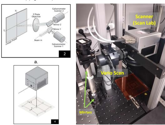
Figure 83. a) Functioning principle of the SCAN Lab system. b) Positioning and image field of the SCAN Lab system. c) Optical scanner system (SCAN Lab) with variable focus system (Vario Scan) in order to change to focus plane of the scanner and change the size of the laser spot.
