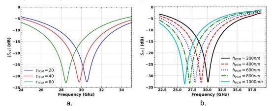
Figure 57. a) Simulation of the variation of the stub's resonant frequency as a function of the permittivity of the GeTe layer. b) Simulation of the variation of the resonant frequency of the stub as a function of the GeTe layer thickness.
