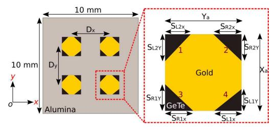
Figure 106. Array of antenna integrating GeTe with asymmetric trimmed edges.
