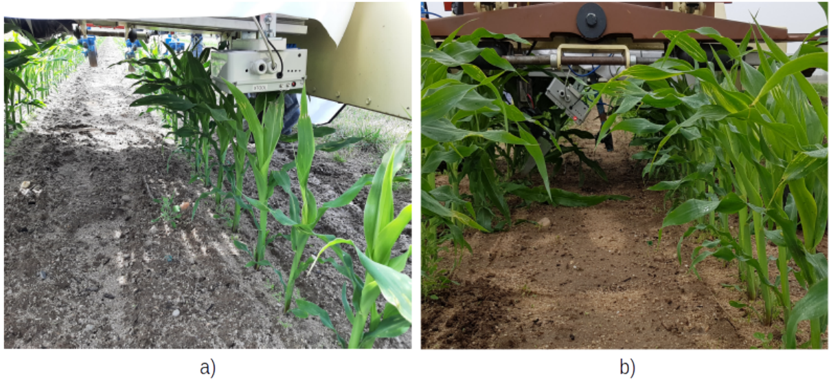
Figure 4.8: Xtool multimodal sensor. a) Obstruction of image acquisition. b) Xtool repositioning.
