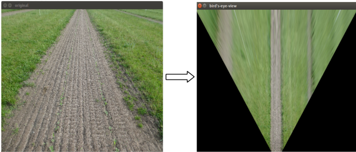
Figure 3.11: Bird's-eye view transformation (on the right) of the image given by the frontal sensor (on the left).
