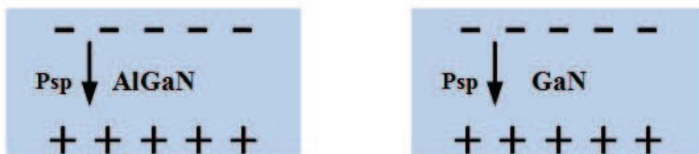
Figure I.19: Spontaneous polarization induced surface charges in the AlGaN and GaN structure.([14])
