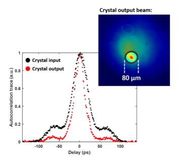
Figure 64: Pulse reshaping observation, by spatially filtering the soliton with a hole (diameter at  $1/e^2 = 80 \mu m$ ). Calculated pulse profiles from the recorded autocorrelation traces. The pump intensity is equal to 0.7 GW/cm², the linear input SOP is 53° and the crystal is at phase matching conditions.
