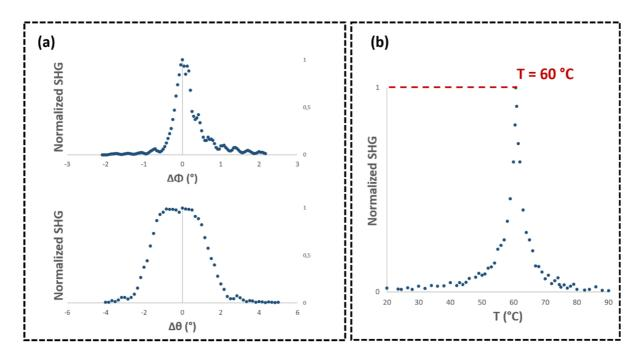
Figure 28: Phase matching curve for: (a)-KTP crystal within horizontal ( $\theta$ ) and vertical ( $\Phi$ ) axis orientation, (b)-PPLN, by modifying the crystal temperature.
