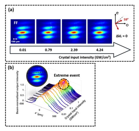
Figure 60: Solitons evolution, on a modulated pump, function of the pump intensity. (a)-FF beams images.
