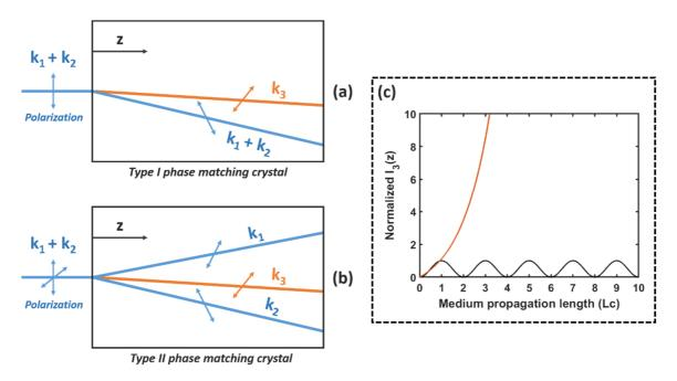
Figure 19: (a)-Example of type I phase matching propagating waves.  $k_1$  and  $k_2$  are the propagating vectors of the incident waves, and  $k_3$  is the propagating vector of the converted wave. (b)-Example of type II phase matching propagating waves. (c)-Normalized generated wave intensity along the birefringent crystal (type I and type II). Black curve is in the case of phase mismatch, and orange curve in the case of phase matching.
