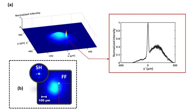
Figure 30: Output spatial beam self-trapping in KTP, for an injected pump intensity of 0.5 GW/cm<sup>2</sup>. (a)-3D view of FF beam, and transverse beam profile of the FF (red inset). (b)-2D representation of the FF and SH beams (SOP set close to 45°,  $\Delta k = 0$ ). The round inset image has the same scale than the square image.
