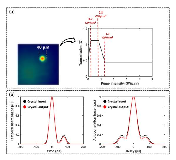
Figure 62: **(a)**-Nonlinear transmission curve obtained by filtering the self-trapped beam with a hole of 40  $\mu$ m of diameter. **(b)**-(Left curve) temporal pulse profiles before and after the temporal filtering; (Right curve) corresponding autocorrelation traces of the two pulses. The figures are obtained at phase matching conditions, with a linear input SOP of 47°.
