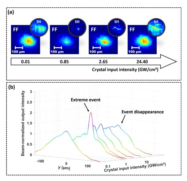
Figure 45: **(a)**-2D output beam images of the FF and SH beams at the end face of the PPLN versus the input pump intensity (the round inset images have the same scale than the square images). **(b)**-1D output profiles evolution of the FF beams versus the input pump intensity. The linear input SOP is set parallel to the crystal extraordinary axis. Positive phase mismatch configuration (21.5 °C).
