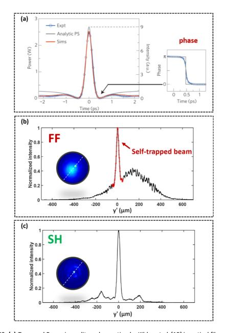
Figure 43: **(a)**-Temporal Peregrine soliton observation by Kibler *et al.* [15] in optical fibers. **(b)**-My observation of the spatial FF soliton. **(c)**-My observation of the SH trapped beam. In both **(b)** and **(c)**, the round insets are the images of the corresponding beams, out of the KTP, and the dashed line in those insets shows the sense of cut for the profile plotting. Phase matching conditions, linear input SOP = 53° and input pump intensity = 0.3 GW/cm<sup>2</sup>.
