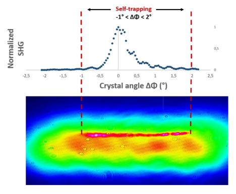
Figure 37: Output images of the FF beam versus the vertical angle  $\Delta\Phi$  of the KTP crystal. **(top)-**SHG curve versus vertical crystal angle of the KTP, **(bottom)-**2D output spatial image of the beam at the end face of the crystal (input pump intensity = 0.3 GW/cm², linear input SOP set close to 45°).
