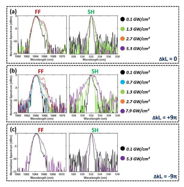
Figure 41: Output spectrum of the trapped beam versus the pump intensity, for a linear input SOP of 69°. (a)- $\Delta kL = 0$ . (b)- $\Delta kL = 9\pi$ . (c)- $\Delta kL = -9\pi$ .
