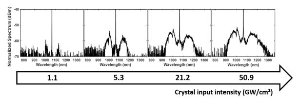
Figure 52: Spectral broadening evolution versus pump intensity, around the FF. Such experimental results are at the phase matching conditions. The linear input SOP is set parallel to the crystal extraordinary axis.
