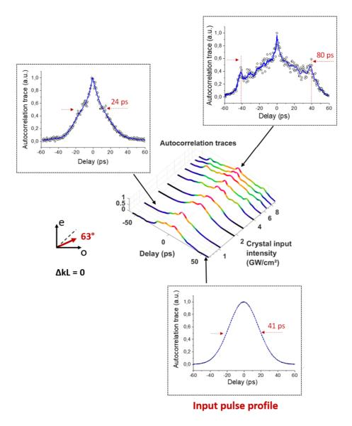
Figure 38: Experimental results of the spatial trapping influence on the temporal domain. Autocorrelation traces of the trapped beam versus the input intensity for  $\Delta kL = 0$  (phase matching) and a linear input SOP = 63°.
