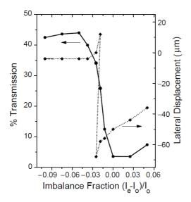
Figure 25: Soliton spatial switching obtained by Torruellas  $\it et~al.$  [63]. They launched a 20 GW/cm² pump into a 1 cm KTP crystal. The solid curve shows the output light transmission at the fundamental frequency through a 30  $\mu$ m aperture (numerical analysis), function of the imbalance between e and o crystal neutral axes. The dashed curve shows the output SH position.
