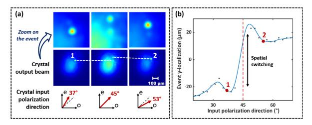
Figure 34: Position of the self-trapped beam versus the linear input SOP (input pump intensity: 0.66 GW/cm² and phase matching conditions). (a)-2D images of the output beam, for three different values of SOP.
