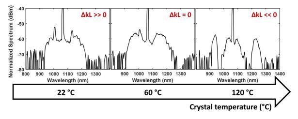
Figure 54: Beam spectral evolution, function of crystal temperature i. e. ΔkL. The pump intensity is of 24.4 GW/cm². The linear input SOP is set parallel to the crystal extraordinary axis.
