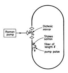
Figure 6: Raman Stokes soliton generation in a fiber cavity [47].
