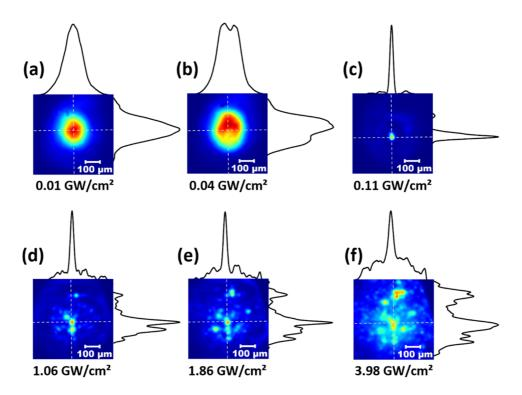
Figure 46: Image of the SH beam, after propagation in the KTP, versus the FF pump intensity.  $\Delta kL = 2\pi$  and linear input SOP of 47°.
