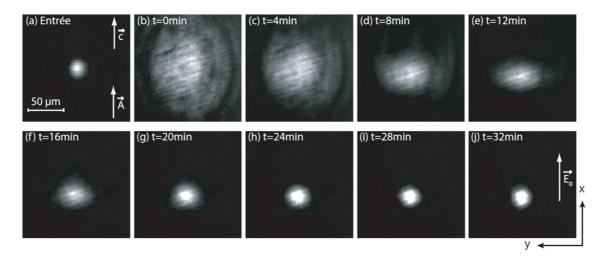
Figure 5: Experimental photorefractive soliton formation in LiNbO<sub>3</sub> material [42]. **(a)**-Input beam shape. **(b-j)**-Output beam shape at different light exposure times. A and C vectors are relative to the optical polarization field, while E<sub>0</sub> vector is relative to the electrical field around the material. The light illumination remains constant during all the process time.
