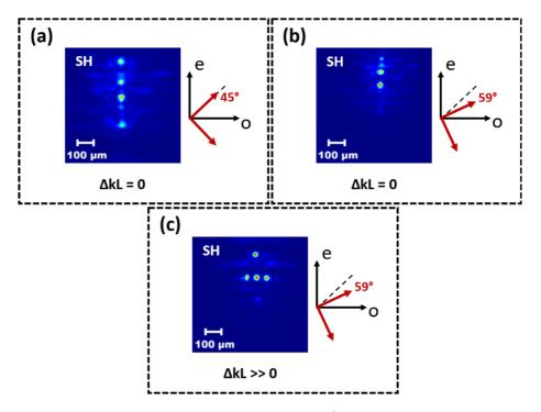
Figure 61: Solitons at the SH for a pump intensity of 0.53 GW/cm<sup>2</sup>. (a)-Phase matching and linear input SOP = 45°. (b)-Phase matching and linear input SOP = 59°. (c)-High positive phase mismatch and linear input SOP = 59°.
