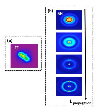
Figure 57: **(a)**-S. Carrasco experimental observations [3] at the output face of a bulk crystal (spatial 2D transverse material - 1064 nm). The input peak intensity is 23 GW/cm<sup>2</sup> **(b)**-S. Carrasco SH profiles simulations [3].
