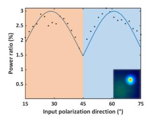
Figure 35: Power ratio between the energy in the confined beam area and the total beam energy, versus the linear input SOP. The input pump intensity is 0.66 GW/cm<sup>2</sup>. All these results have been obtained at phase matching conditions.
