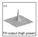
Figure 21: Quadratic soliton observation made by Torruellas [28]. (a)-The input beam. (b)-The output beam at low input light intensity. (c)-The output beam at high input intensity (more than 10 GW/cm²). All of these images are at the fundamental frequency.
