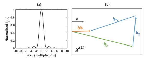
Figure 17: (a)-Second harmonic generation versus the nonlinear medium length and the phase mismatch between the waves involved in the process. (b)-Phase mismatch representation. Where  $k_1$  and  $k_2$  are the propagating vectors of the depleted waves, and  $k_3$  is the propagating vector of the generated wave.
