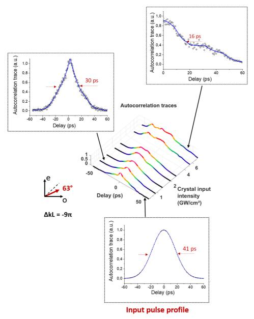
Figure 40: Experimental results of the spatial trapping impact on the temporal domain. Autocorrelation traces of the trapped beam versus the input intensity for  $\Delta kL = -9\pi$  and a linear input SOP = 63°.
