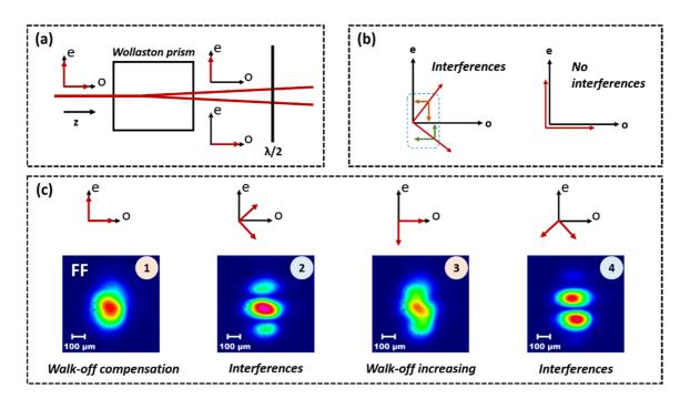
Figure 58: **(a)**-Experimental setup used to convert one beam in two with perpendicular polarization directions. **(b)**-Two different excitations of the crystal leading to spatial interferences and no interferences. **(c)**-Images of the output pattern for different linear input SOP orientation. Phase matching conditions and input pump intensity = 0.01 GW/cm<sup>2</sup>.
