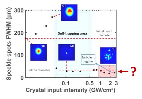
Figure 42: Spatial evolution of the SH beam versus the input intensity. The vertical axis reports the elementary spot diameter constituting it ( $\Delta kL = 2\pi$  and linear input SOP ~ 45°).
