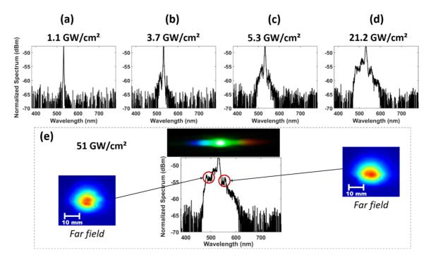
Figure 51: (a-d)-SH beams spectral evolution, for different pump intensity values. (e)-SH beam spectrum for an input pump intensity of 51 GW/cm<sup>2</sup> and corresponding beam images. Both insets are the far-field beam images at 500 nm (left) and 550 nm (right), respectively. Such experimental results are at the phase matching conditions. The linear input SOP is set parallel to the crystal extraordinary axis.
