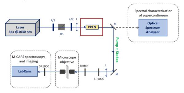
Figure 66: M-CARS experimental setup, with a PPLN and without delay line, realized by S. Wehbi *et al.* at XLIM laboratory [19]. **\( \lambda/2:** half-wave plate, **BS:** polarizing beam splitter, **L:** lens, **M:** mirror, **SP1000:** short-pass filter (<1000 nm), **LP1000:** long-pass filter (>1000 nm).
