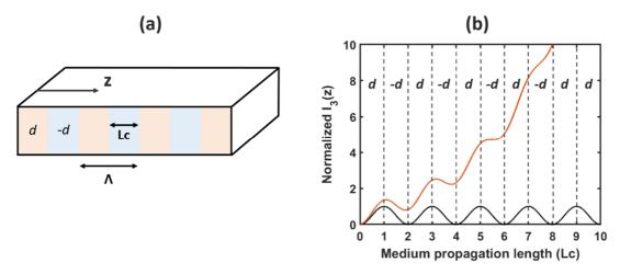
Figure 20: **(a)**-Poled crystal with  $\Lambda = 2L_c$  period. **(b)**-Normalized intensity of the generated third wave along the crystal. Black curve is in the case of phase mismatch, and orange curve in the case of quasi-phase-matching.
