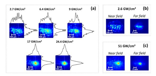
Figure 50: **(a)**-Near-field images of the PPLN output SH beam, for different values of pump intensity. Near and far fields of the SH for **(b)**-Pump intensity = 2.6 GW/cm<sup>2</sup>, **(c)**-Pump intensity = 51 GW/cm<sup>2</sup>. Such experimental results are at the phase matching conditions. The linear input SOP is set parallel to the crystal extraordinary axis.
