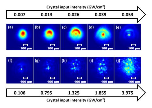
Figure 32: 2D representation of the SH beam evolution versus the input intensity. Phase matching conditions, linear input SOP set close to 45°. Images from (a) to (j) are for different input pump intensities.
