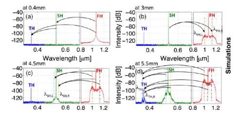
Figure 53: Numerical simulation of the spectral evolution along the propagation length of a PPLN crystal. L and R are respectively the anti-Stokes and the Stokes waves. Phase mismatch conditions ( $\Delta kL = -3\pi$ ), and pump intensity = 1 GW/cm<sup>2</sup>. This figure is extracted from Ref [10].
