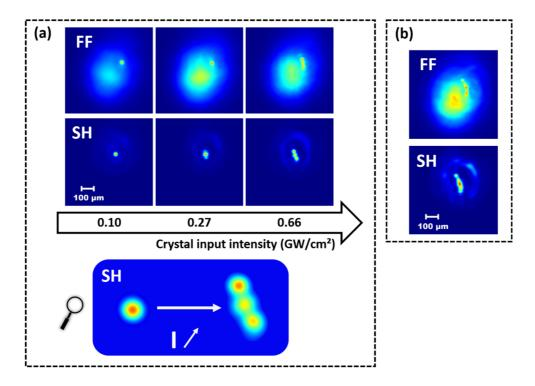
Figure 56: Multiple quadratic solitons observation. Images of the output FF and SH beams for three different input intensities,  $\Delta kL = 9\pi$ , input linear SOP at 47°. (a)-Evolution of the pump intensity from 0.1 to 0.66 GW/cm². (b)-Pump intensity = 1.1 GW/cm².
