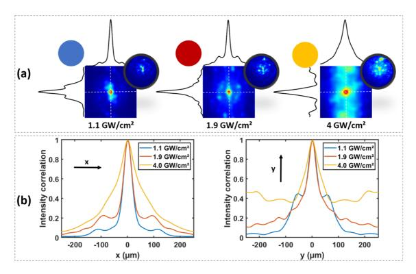
Figure 49: **(a)**-Intensity correlations  $C_1$  of the near-field SH images. **(b)**-Comparison of each intensity correlation spatial profiles, cut on x or on y transverse axes.  $\Delta kL = 2\pi$  and linear input SOP of 47°.
