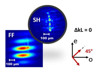
Figure 59: Soliton on a modulated pump. The FF and SH beams images are for an input pump intensity of 0.66 GW/cm<sup>2</sup>. Phase matching conditions and linear input SOP = 45°.
