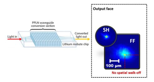
Figure 44: **Left-**Schematic of a PPLN crystal. **Right-**Spatial output soliton after propagation in the PPLN, excited by a collimated beam (positive phase mismatch i. e. crystal temperature = 21.5 °C), and input pump intensity = 0.85 GW/cm<sup>2</sup>). The linear input SOP is set parallel to the crystal extraordinary axis. The round inset image has the same scale than the square image.
