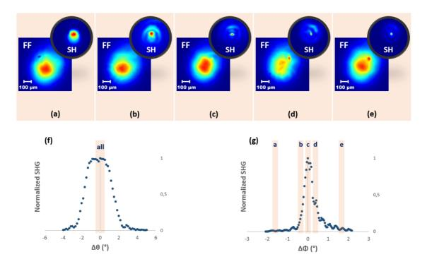
Figure 55: Profile of the output FF and SH beams versus the phase mismatch and for an input linear SOP of 47° and an input pump intensity of 0.05 GW/cm². (a)- $\Delta\Phi$  = -1.67° ( $\Delta$ kL = -9 $\pi$ ); (b)- $\Delta\Phi$  = -0.33°, ( $\Delta$ kL = -2 $\pi$ ); (c)- $\Delta\Phi$  = 0° ( $\Delta$ kL = 0); (d)- $\Delta\Phi$  = 0.33°, ( $\Delta$ kL = 2 $\pi$ ); (e)- $\Delta\Phi$  = 1.67° ( $\Delta$ kL = 9 $\pi$ ); (f)-Normalized SHG curve versus  $\Delta\Theta$ .
