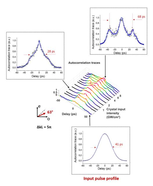
Figure 39: Experimental results of the spatial trapping impact on the temporal domain. Autocorrelation traces of the trapped beam versus the input intensity for  $\Delta kL = 5\pi$  and a linear input SOP = 63°.
