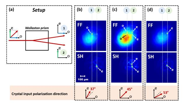
Figure 36: Polarization content of the self-trapped beam versus the linear input SOP. (a)-Schematic representation of the system used to realize the experiment; (b-d)-2D spatial output images for three different polarization states and for both FF (top) and SH (bottom) beams (Intensity: 0.66 GW/cm², phase matching conditions).
