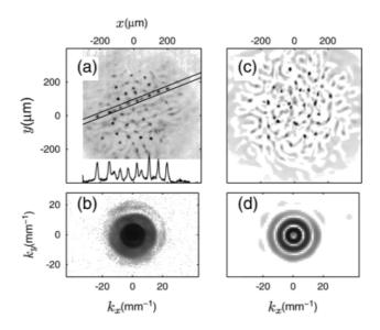
Figure 24: 2D MI observed by M. Delqué et al. [57]. (a)-Experimental results (10 MW peak power) and (b)-Corresponding spatial spectrum. (c)-Simulation (10 MW peak power) and (d)-Corresponding spatial spectrum.
