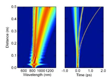
Figure 7: Numerical simulation of a supercontinuum generation in an optical fiber, due to N = 3 soliton fission [62]. **Left-**The resulting supercontinuum of light. **Right-**Time shift of the high-energy solitons while propagating in the fiber, after fission of the injected (Distance = 0) soliton.
