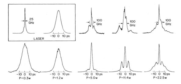
Figure 2: First temporal soliton recorded by Mollenauer *et al.* [9]. For various fiber input powers, the figure illustrates the spectrum and temporal traces of the output fiber beam (the temporal traces are from an autocorrelation and the curves are normalized). The box shows the input laser characteristics.
